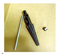
The 2044R Tie-Rod Flip Kit includes a Reamer and a Knuckle Tapered sleeve Insert. The insert is shown on right and the reamer to be used is on the left.
