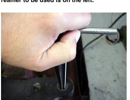
4 Gently turn the reamer clockwise to remove material from the topside of the knuckle as shown above.
