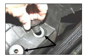
**9.** Install the 2 well nuts (#18) into the holes in the plastic air cleaner mount where you removed the grommets in step #6.
