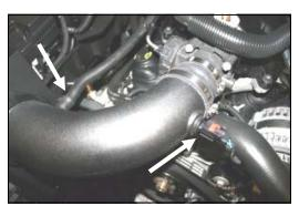
17. <u>Very Carefully</u> reinstall the temperature sensor removed in step #1, into the grommet in the Airaid Intake Tube, and then reconnect the wiring harness. Reconnect the factory breather hose to the nipple on the intake tube, and install the supplied speed clamp (#19) over the hose.
