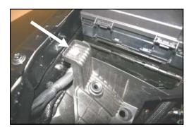
**7.** Using a 10mm socket, remove and save the bolt from the factory plastic air cleaner mount. It will be re-installed in step #12.
