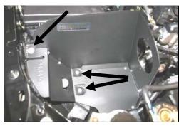
12. Install the CAD into the vehicle. Install the two 3/8x1" button head bolts (#13), thru the bottom panel, and into the well nuts. Reinstall the factory bolt removed in step #7 thru the panel, and into the fender well. Tighten all three bolts at this time.
