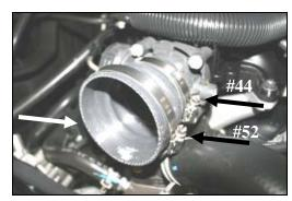
**15.** Install the reducing hump hose (#5) onto the throttle body as shown, with the #44 hose clamp (#15) on the back, and the #52 hose clamp (#16) on the front. Leave the clamps loose for now.
