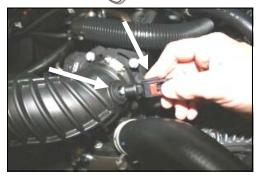
1. **Disconnect the negative battery cable.**Disconnect the wiring harness connected to the air temperature sensor. **WARNING!** Electrical connector & sensor are very fragile. **USE CAUTION! Very Carefully** remove the temperature sensor from the factory intake tube by using a small circular motion while pulling it straight out.
