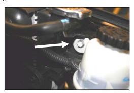
**8.** Using a 10mm socket, remove and save the bolt that holds the radiator to the radiator support. It will be reused in step #10.
